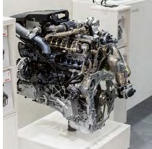
General Motors' 3.0-l Duramax diesel inline six-cylinder engine (© ÖVK | Klaus Ranger)
